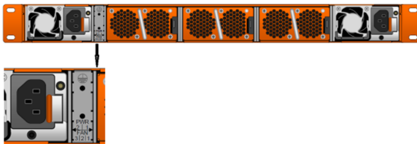
Figure 8 Holes for Ground Screws
